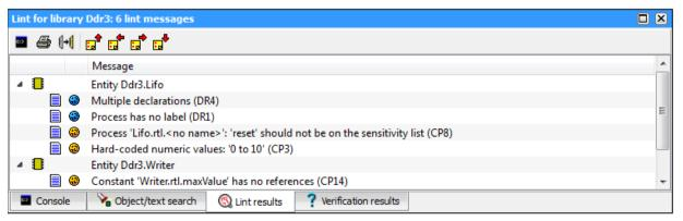
design scalability and quality. The linting is based on the DO-254 'Best Practice Design Rule Set'. The messages are hot-linked to the corresponding editor so you can quickly navigate to the offending code.
