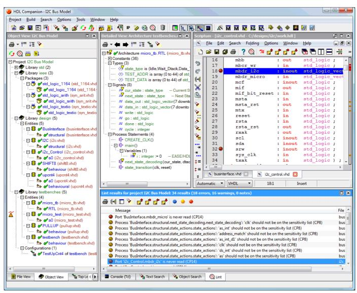
In the past a designer had to use a simple text editor and Unix like 'grep' commands to find his way through many lines of HDL code or use a costly simulator license to understand the design structure. With HDL Companion a designer can drag and drop design files or directories into the file view and a complete design decomposition is performed in seconds, offering information regarding numerous aspects of the design.
