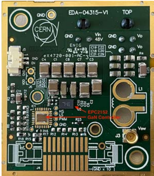
Fig.1: bPOL48V board hosting GaN_Controller and EPC2152.
