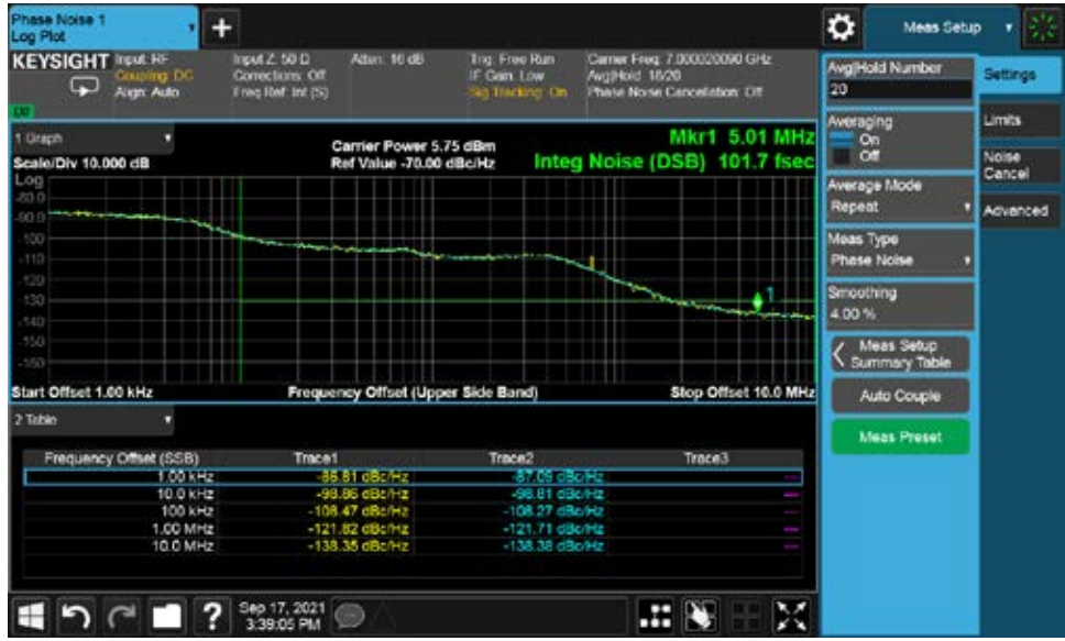
Fig2. PLL 7GHz measured performance with reference operating at 200MHz (2 X 100MHz external reference).
